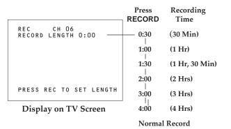
The REC and TIMER indicators light in the VCR's display panel. During recording, press RECORD on the VCR or REC on the remote to display the time remaining on the TV screen. Press RECORD or REC again to increase the recording time.
